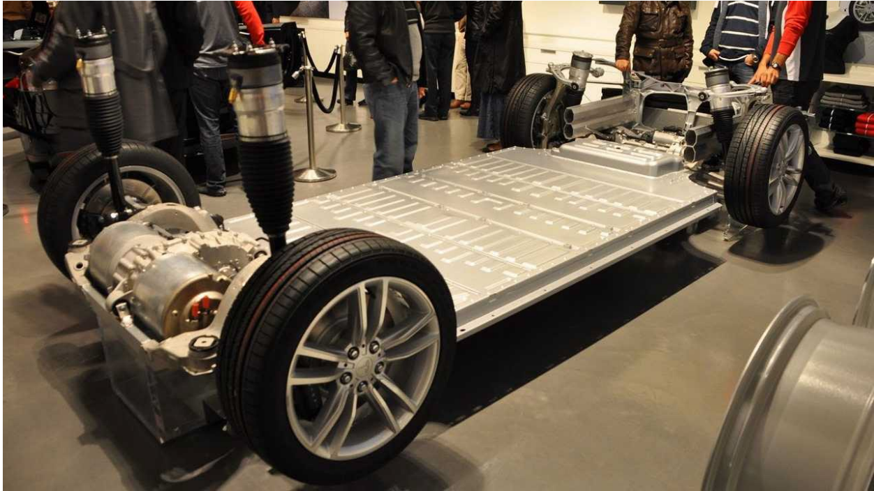
Figure 24 One example of the BEV skateboard design. Source: https://insideevs.com/news/450534/tesla-leaves-skateboard-design-new-structural-battery-packs/
